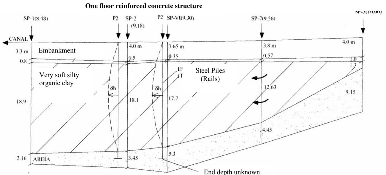
Figure 13. Geotecnical profile – horizontal pull
