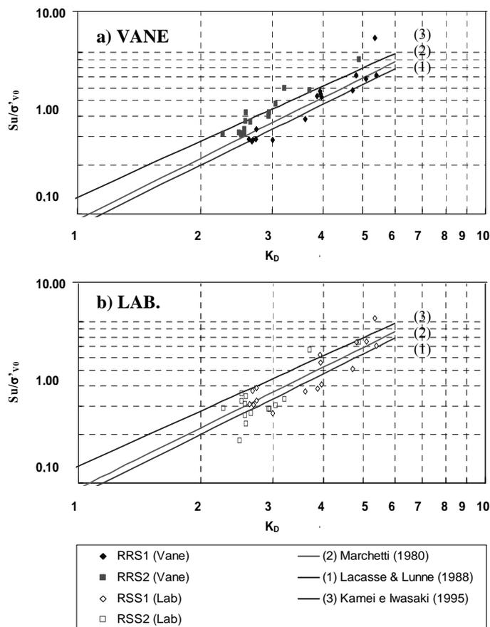
Figure 12.  $S_u$  vs.  $K_D$  parameters: (a) Vane Test; (b) Laboratory test – TC.
