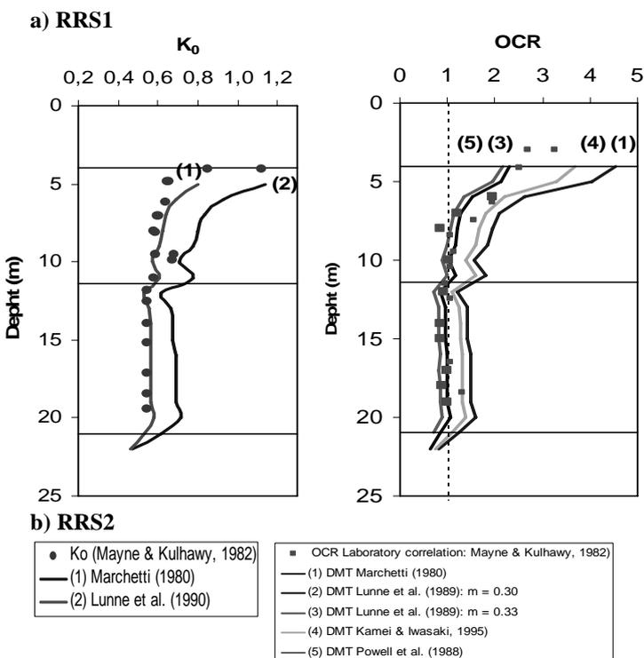
Figure 6. Stress history and in situ horizontal stress parameters: (a) Research Site 1; (b) Research Site 2.
